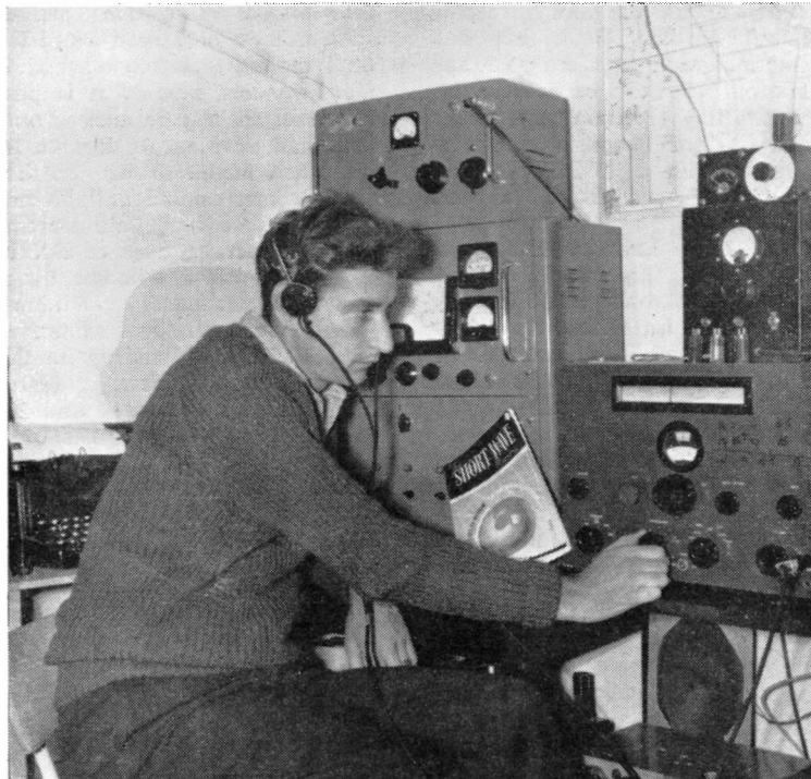
G3PQC is operated by D. Turk, 25 Whetstone Road, Cove, Farnborough, Hants., who was licensed at Christmas 1961. He started out on Top Band before building an all-band Tx based on a Geloso VFO unit. His receiver is a CR-100 and the present aerial is a 67 ft. doublet. Operation is CW, mainly on 160-40-20 metres. G3PQC, who is a member of the Royal Naval Amateur Radio Society, would like to hear from any R.N. types who recognise him here.
